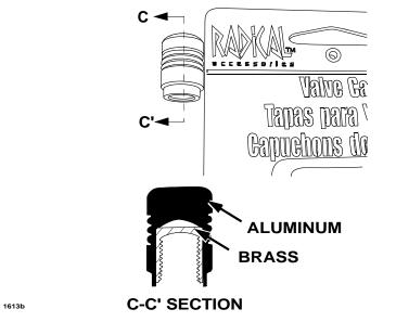
This service tip is to aid in informing customers of the damage that may be caused to the TPMS wheel units by installing these types of valve step caps. When you encounter this concern, please advise the customer to use aluminum or plastic caps ONLY. Also, ensure that the caps they choose to install DO NOT have a brass thread insert.
