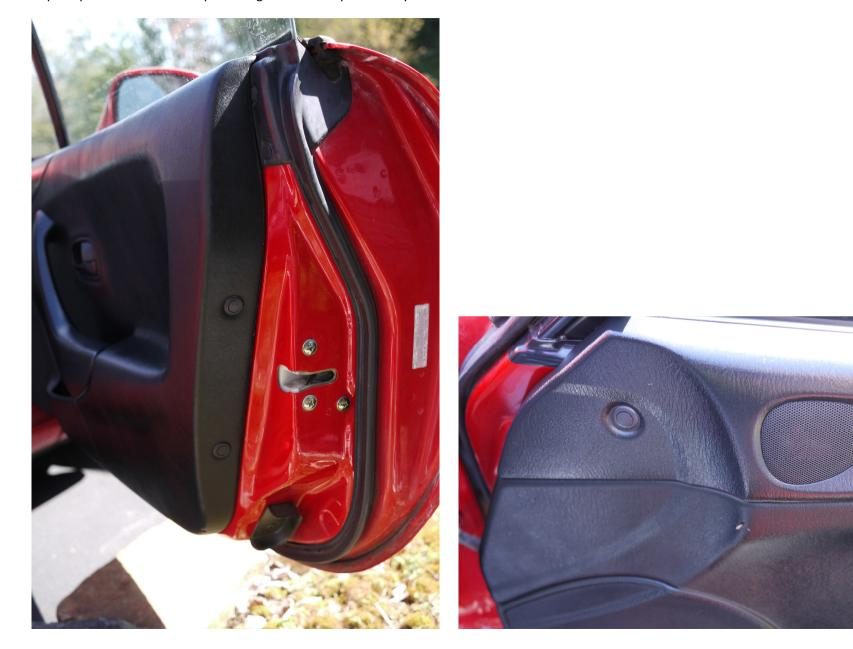
There are three (3) Philips head screws that need to be removed as well.
