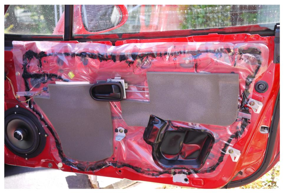
Begin to peel the vapor barrier back like so and lower the window down. Take note of window position.
