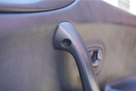
Insert a nylon pry bar between the door panel and door about the perimeter. Take care of the speaker. When the door panel is loose, grasp the pull of the inner door panel firmly and wiggle up. Set the door panel aside.
