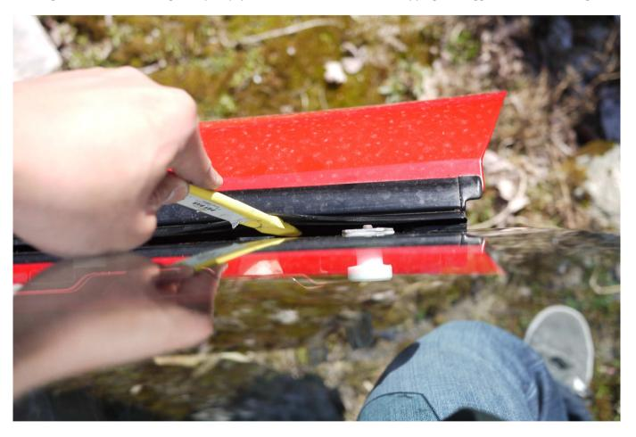
More, an impression is left on the plastic pieces, glass and sheet metal of where the hardware originally was. Use them to aid in reinstallation. The difference after is incredible. Hope this helps somebody out there.
