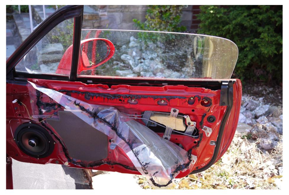
This permits 2 of the 3 screws which hold the window in place to be removed through the opening of the door.
