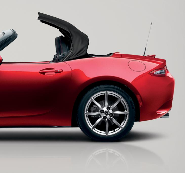
Our first-ever ingenious power retractable roof operates in a mere 13 seconds. Press a button and the fastback side pillars raise, the two overhead roof panels retract, and the rear window lowers itself behind the seats. The two fastback pillars return into place to retain the sleek fastback style.
