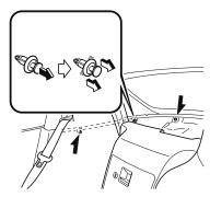
4. Push the stopper rubber through the cover on the right side of the vehicle while slightly lifting the cover up.
