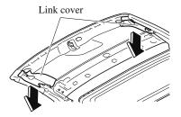
5. Remove the fasteners and the headliner.
