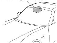
The Forward Sensing Camera (FSC) determines the conditions ahead of the vehicle while traveling at night and detects traffic lanes. The distance in which the Forward Sensing Camera (FSC) can detect objects varies depending on the surrounding conditions.
