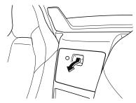
To open, press the latch down to open the seat side box.
