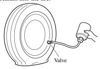
12. Pull out the injection hose from the valve.
