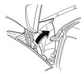
8. Insert your hand beneath the lifted cover and loosen the cap screws until they spin freely.
