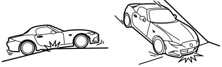
This vehicle is equipped with low profile tires allowing class-leading performance and handling. As a result, the sidewall of the tires are very thin and the tires and wheels can be damaged if driven through potholes or on rough/uneven roads at excessive speeds. Use care and reduce speed when traveling on rough/uneven roads or through potholes.
