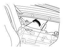
14. Pull out the cap and release the trunk lock.
