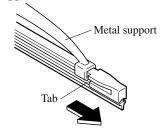
3. Remove the metal stiffeners from each blade rubber and install them in the new blade.
