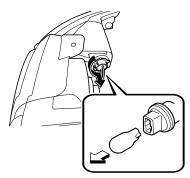
12. Install the new bulb in the reverse order of the removal procedure.
