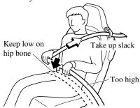
Before fastening the seat belt, make sure that the seat belt passes through the seat belt guide correctly and it is not twisted.
