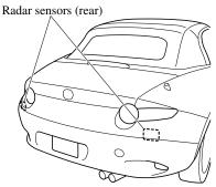
The radar sensors (rear) are installed inside the rear bumper, one each on the left and right sides.
