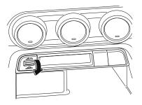
Pour about 200 ml (200 cc) of water at once into each of the left and right drainage outlets to wash away small particles of foreign matter inside the drainage path.
