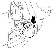
3. Remove drain filter B out of the opening after removing drain filter A.
