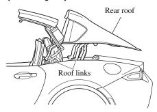
After cleaning the drainage outlets, continuously press the retractable hardtop switch in the close direction to close the rear roof. Refer to Closing the Roof on page 3-44.
