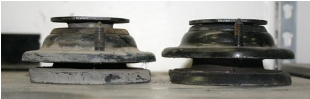
COLLAPSED SHOCK MOUNT ON LEFT
