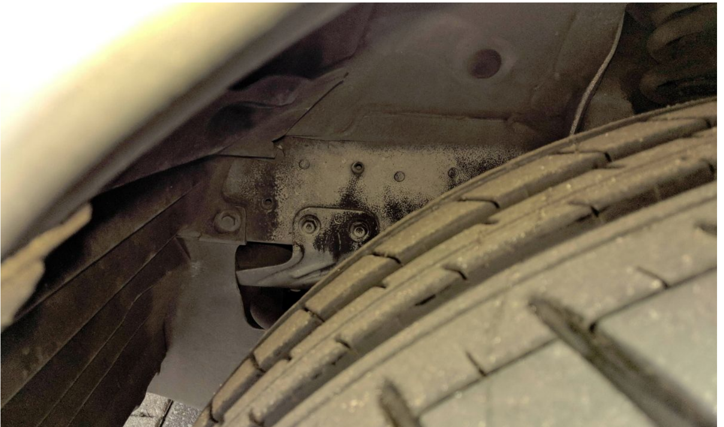
NB FRAME RAIL INTACT (NO RUST)
