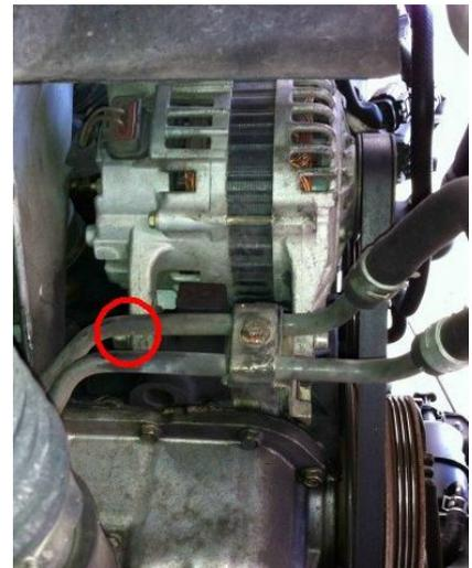
Use a 14mm wrench to loosen bolt 2. Get up and dust yourself off. Loosen bolt 3 with a 12mm socket to move the alternator. If you just want to tighten this belt, then skip down to the next page. Slip off the belt.
