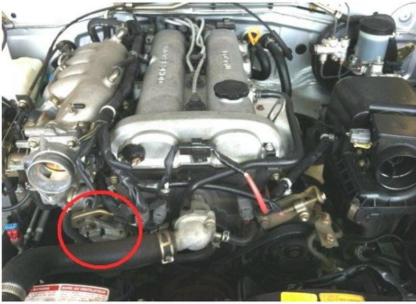
The second belt goes from the engine to the water pump pulley above then the alternator. The tension in this belt comes from the alternator compressor pulley. The tensioner (circled) needs to be adjusted to remove the belt.
