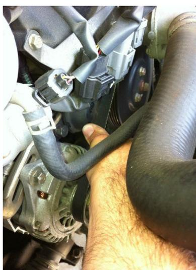
Put the new belt on the alternator loop. First wrap it around the water pump pulley, then the engine pulley (the groove closest to the engine) and lastly around the alternator. As you tighten bolt 3, check the tension on the belt with your *calibrated* finger. The belt need to be tightened so that 22 lbs causes 1/3 inch deflection. If you don't trust your finger, then you can get a belt tension gauge like the one to the right.
