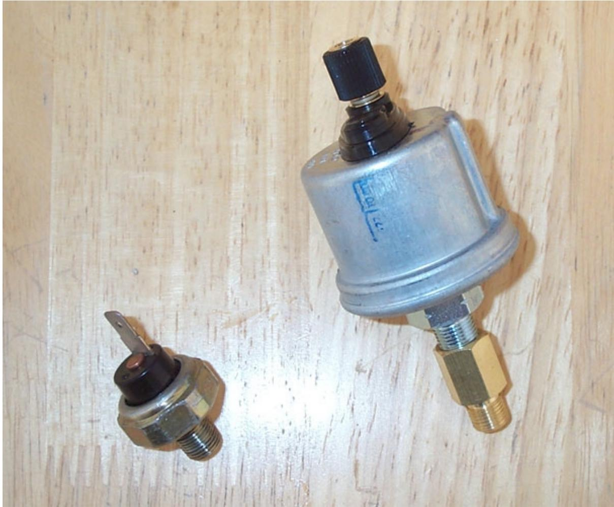
The oil pressure sender is on the right side of the engine above the oil filter. It's a pain to get to from all angles. I ended up cutting my wheels to the left and reaching in from behind the passenger wheel. This is only possible if you have long arms. A 24mm deep socket is ideal for removing the old oil sender switch. I have a 1-1/8" and 1" oil sender sockets and the 1" socket was too large. When unscrewing the old sender, about 2 tablespoons of oil will leak out, be ready to catch it.
