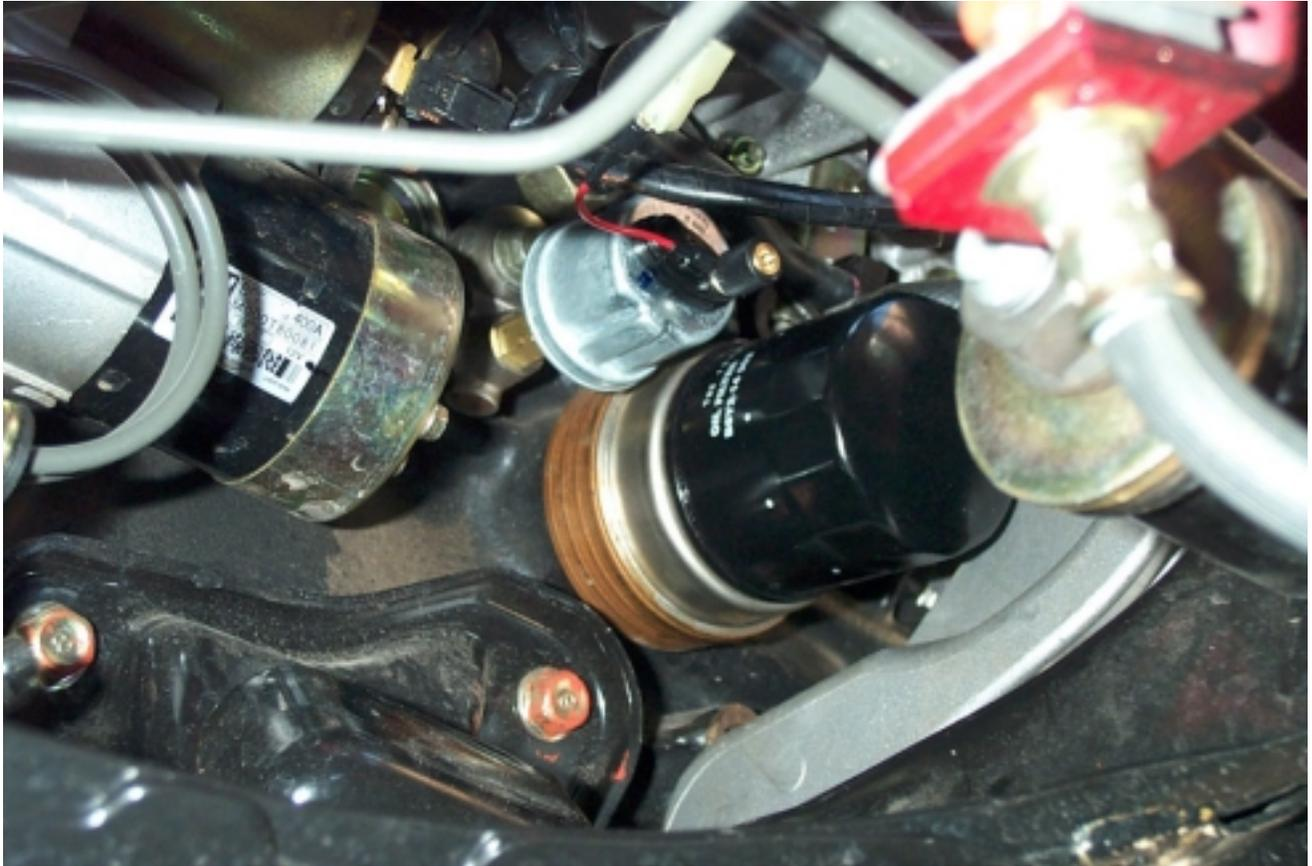
The VDO sender doesn't have the same press-on connector that the OEM sender has, so I built a short adapter cable to use. You could cut the original connector off, but that's hardly professional.
