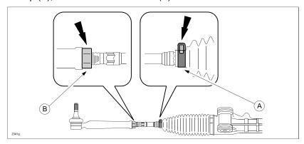
3. Rotate the tie-rod to adjust the steering wheel center. Refer to the following charts for rotating direction.
