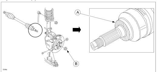
4. Apply molybdenum grease onto the drive shaft and wheel bearing mating surface (A).
