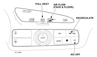
**NOTE:** There are three A/C positions on the LCD panel (A/C, A/C econ, <blank>). Depress the A/C button until <br/>blank> is selected.
