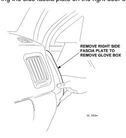
3. Remove the six (6) phillips screws to remove the glove box assembly.
