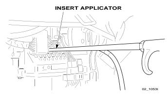
5. Spray the entire contents of the bottle in short bursts, 3 seconds ON, 3 seconds OFF into the rotating fan. A fine mist may exit from the ducts.
