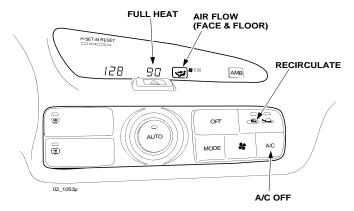
**NOTE:** There are three A/C positions on the LCD panel (A/C, A/C econ, <blank>). Depress the A/C button until <br/>blank> is selected.
