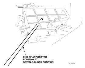
5. Spray the entire contents of the bottle in short bursts, 3 seconds ON, 3 seconds OFF into the rotating fan. A fine mist may exit from the ducts.
