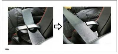
To correct the problem, the shape of the seat belt guide has been changed.
