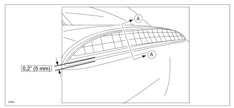
Explain to the customer that water (A) becomes trapped under the lower edge of the lens (B) and the inside of the light assembly is not getting wet. To remove the water drops temporarily, allow the high mount stop light to dry or blow the water drops off using compressed air (C).
