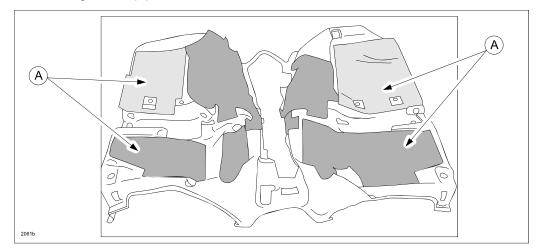
3. Clean bottom of carpet to ensure new felt adhesive attaches properly.
