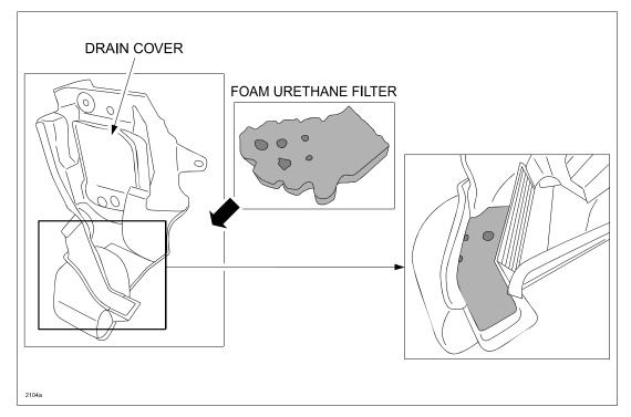
Verify repair by pouring water into the drain covers prior to reassembly to confirming water only exits under vehicle and does not leak from drain valve tubes assemblies into retractor holes and/or overflow drain cover assemblies.
