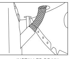
INSTALLED DRAIN VALVE ASSEMBLY
