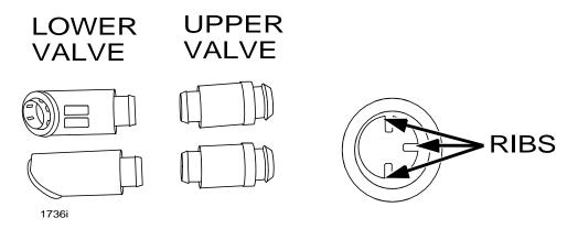
3. Install the modified lower value in the same position as the old value when removed.
