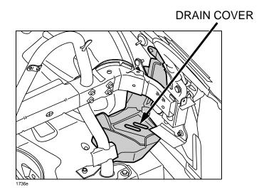
2. To ensure proper adhesion of the filter to drain cover assemblies, wipe down contact area with Isopropyl alcohol.
