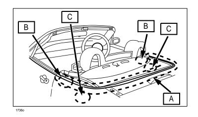
**AREA "B":** Insert the vacuum cleaner hose inside the convertible top, remove leaves and/or debris from top of the drain cover filter on right and left side of vehicle.
