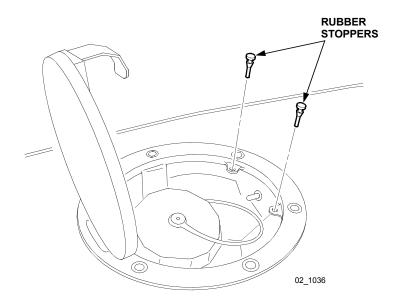
3. Install (2) revised rubber stoppers pushing downwards.
