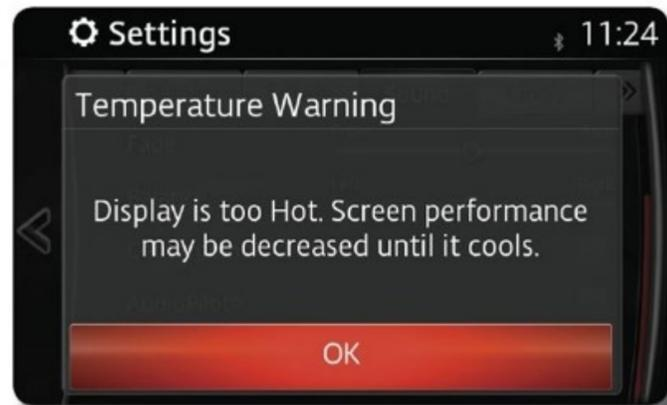
Normal screen operation will resume when the screen temperature cools. If the warning message remains on, have the vehicle inspected at an authorized Mazda Dealer. AGP
