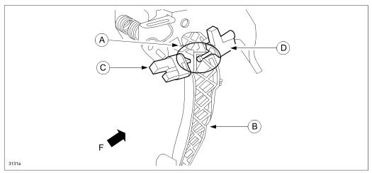
To prevent the stick-slip noise from occurring, two pieces of silicon pad have been attached to the clutch pedal where the two switches contact.
