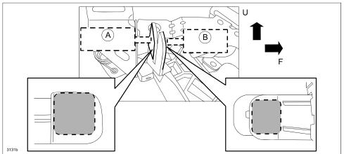
c. Peel off the protective foil and apply the silicon pad to the clutch pedal as shown below (the clutch pedal position switch and the starter interlock switch sides).
