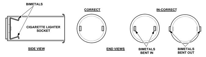
To prevent future concerns, be sure to inform customer of proper usage of power adapters and the necessity of using a cigarette lighter of correct dimensions as shown below.
