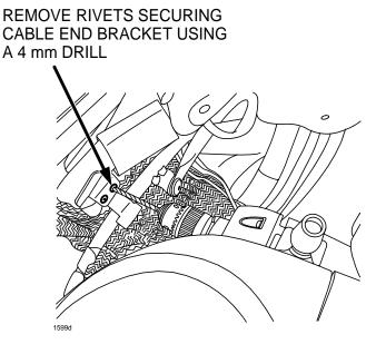
4. Loosen the nut and remove the damaged cable end bracket.
