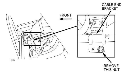
3. Add a washer (1.0 mm – 1.5 mm thick) between the cable end bracket and convertible top frame.
