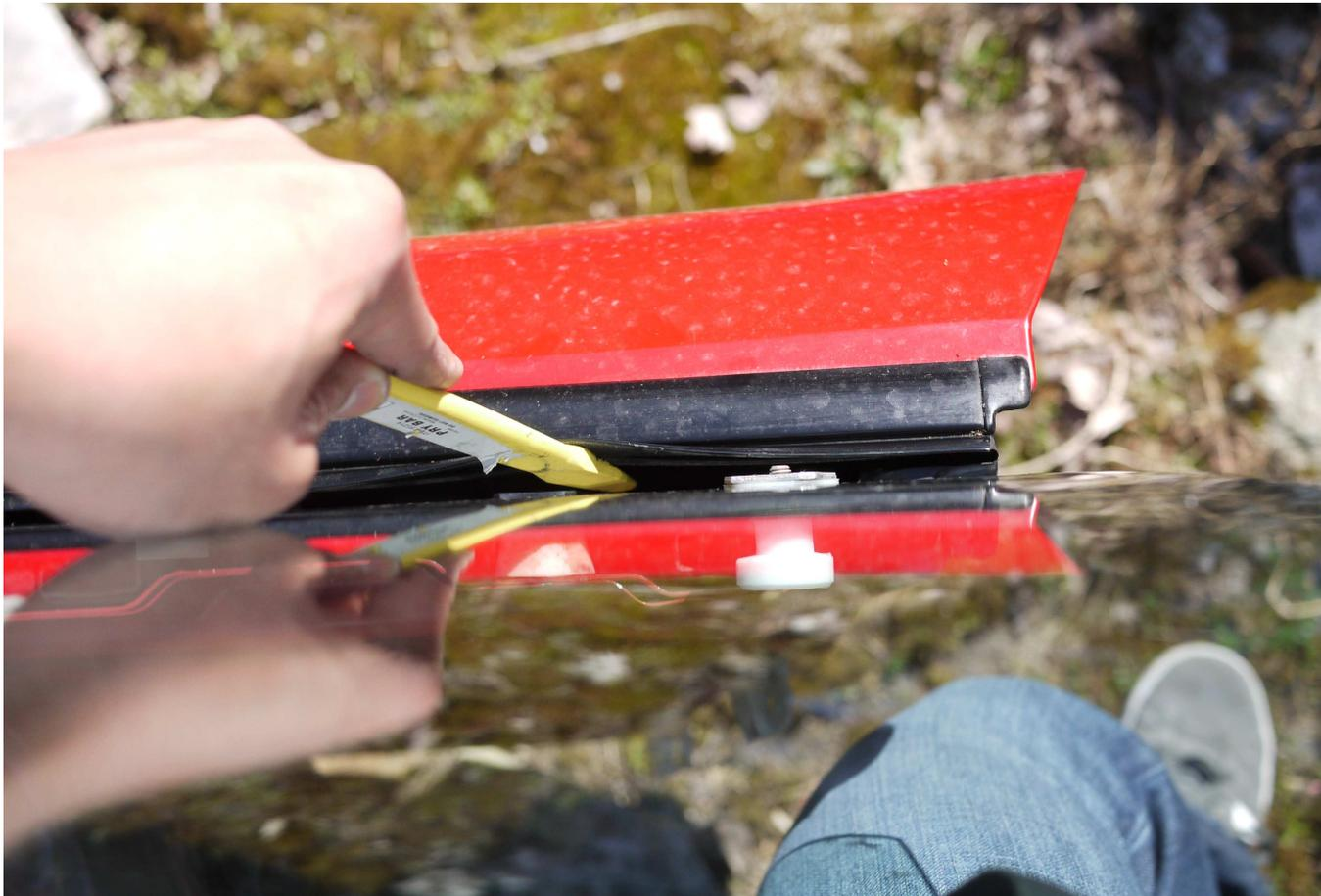
More, an impression is left on the plastic pieces, glass and sheet metal of where the hardware originally was. Use them to aid in reinstallation.
