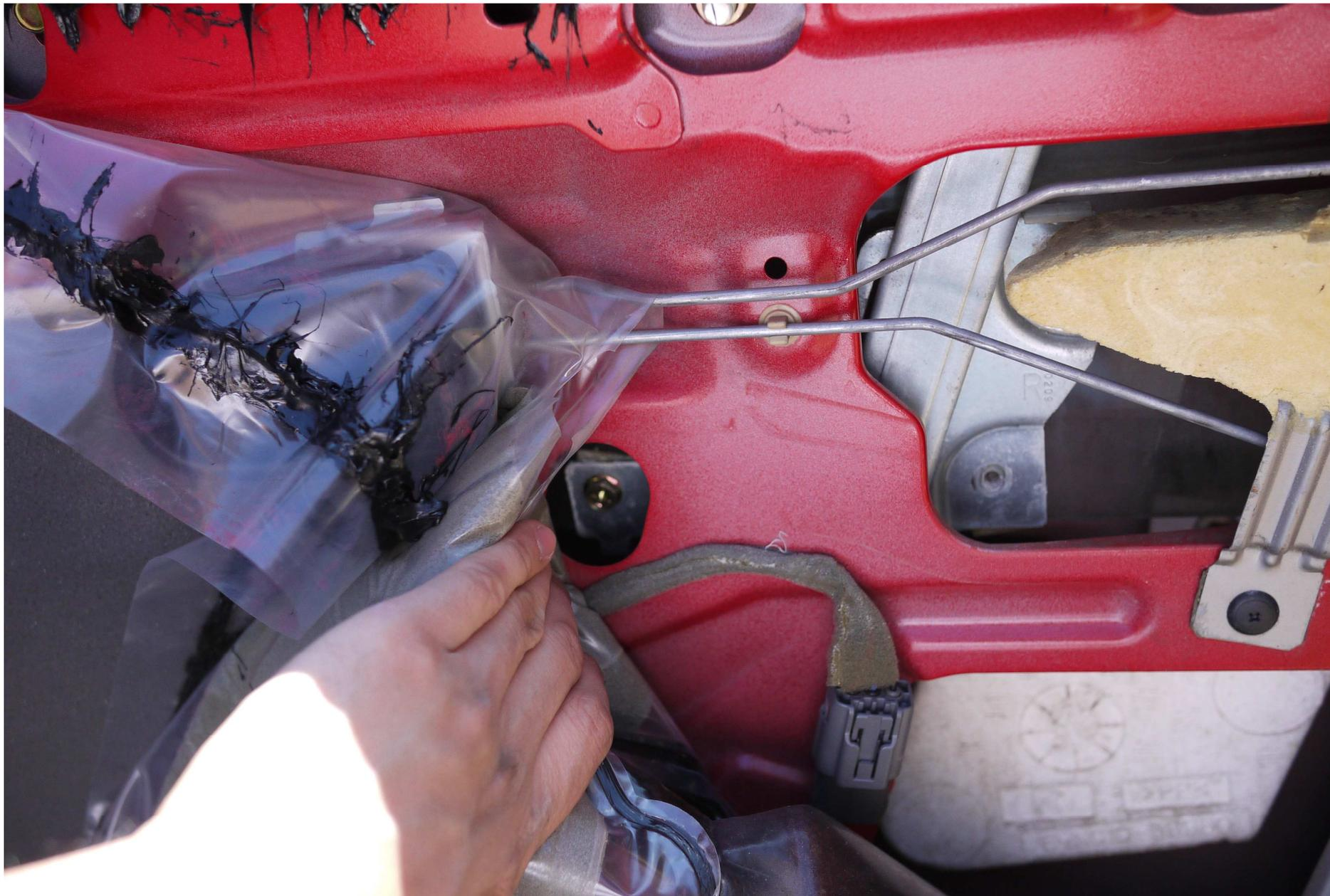
There are also upper window stops that prevent removal of the glass from the door and need to be removed. They dictate when the window stops when closed. I found there were two on the passenger side but only one on the driver side. This procedure covers the passenger side. Slip your fingers alongside of the interior of the glass when removing to keep them from falling and spinning free as they are threaded.
