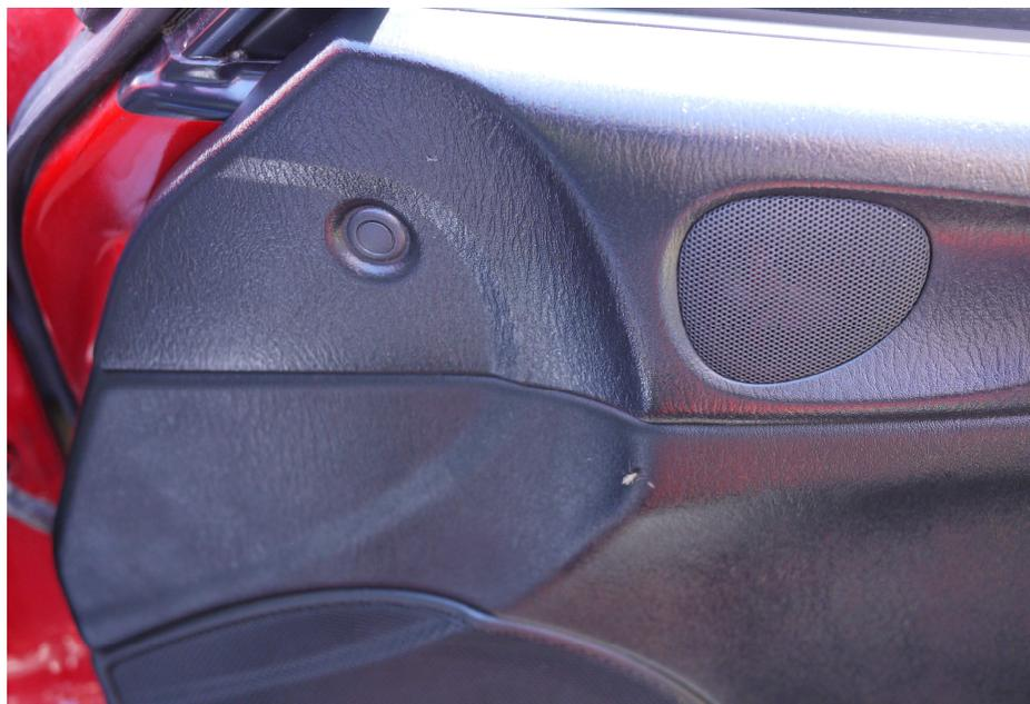
There are three (3) Philips head screws that need to be removed as well.
