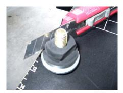
Then cut the secants of rubber bushing with a knife.....
