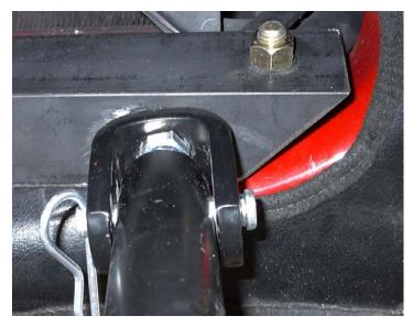
Place the bar in place and tight the nuts until the top of the L-beam makes full contact with the lashing hooks of the Miata.
